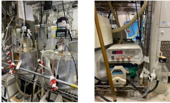
Fig. 2. Two anaerobic fermentation reactors(left) and pH regulator system(right).
