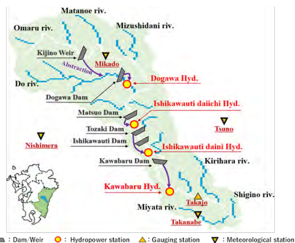
Fig.1 The Omaru River catchment. The main stem and tributaries are depicted by white and blue colors, respectively. Arrows indicate water conveyance from the dams to the hydropower stations.
